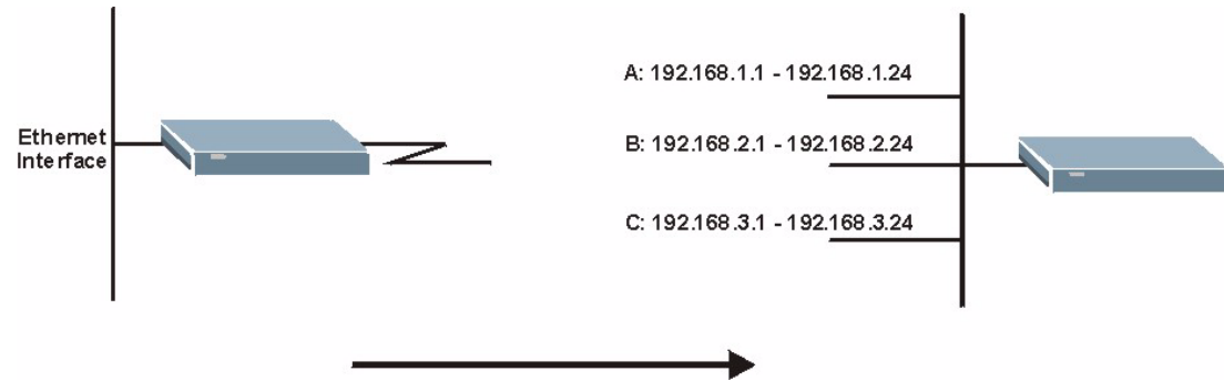
Figure 25 Physical Network & Partitioned Logical Networks
