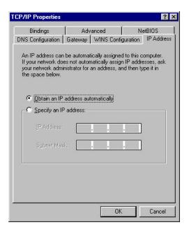
**Step 3.** The **TCP/IP Properties** dialog with **IP Address** tab will appear as shown below.
