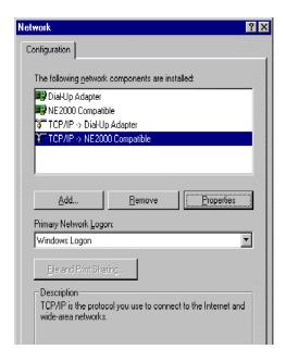
**Step 2.** Double-click the *Network* icon to open the *Network* control panel. A list of installed components is displayed. Click on *TCP/IP* selection for the installed network card to highlight as shown below, then click the *Properties* button.
