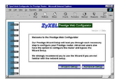
**Step 2.** Click the *Wizard Setup* button at the bottom of the welcome screen to start down the Wizard Setup path.
