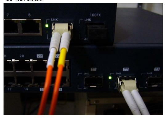
If you connected the cable correctly, the LED of the "LINK" will light up.
