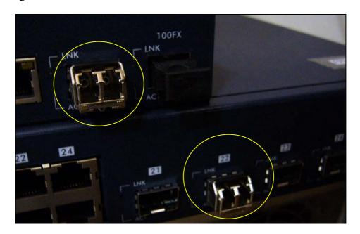
5. Remove both side of the protection cap from the LC/LC Fiber Cable.
