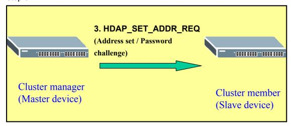
HDAP\_SET\_ADDR\_REQ (Master device) packet request is used for a clustering manager to assign an IP address and subnet mask to a clustering member.
