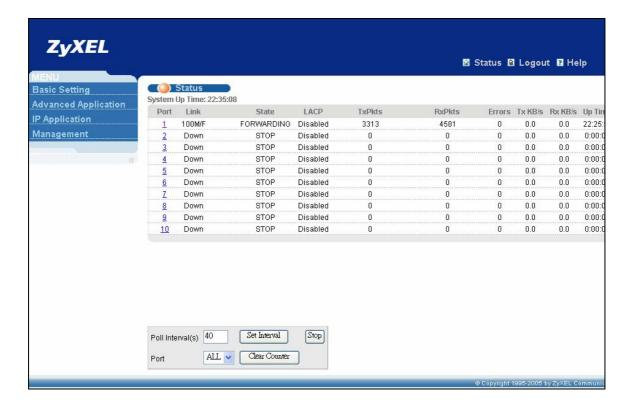
7. First, we need to tell the Switch to run VLAN as port based instead of 802.1q based. In order to do so, we first click on the "Basic Setting", then "Switch Setup"; on your right screen the VLAN Type, choose "Port Based" instead of "802.1Q", and click "Apply" to save your changes.
