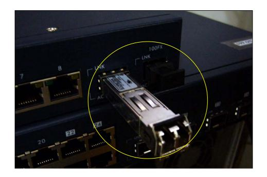
4. Plug another transceiver into the Mini-GB Port of GS-4024 Switch
