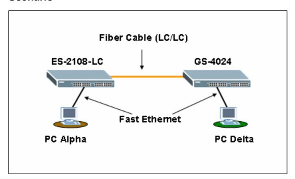
In this scenario, ES-2108-LC is connected to GS-4024 via the mini-GB Port with a LC/LC Fiber cable (62.5/125MM). PC "Alpha" is connected to ES-2108-LC and another PC "Delta" is connected to the GS-4024 Switch via the RJ45 Port.
