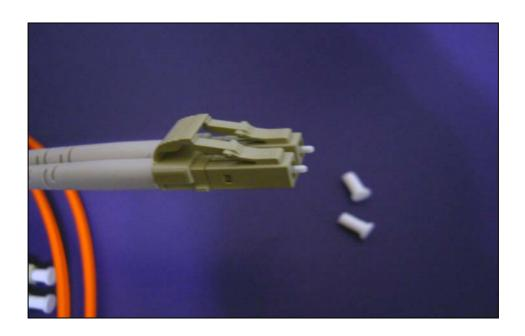
6. Plug the LC/LC Fiber Cable into the transceivers on both ES-2108-LC and GS-4024 Switch.
