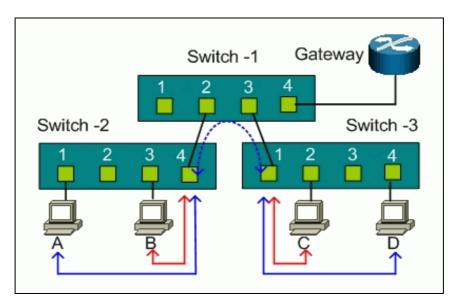
For Switch-2, port 1, port 2, and port 3 are allowed to communicate back and forth with uplink port 4, but not with other ports.
