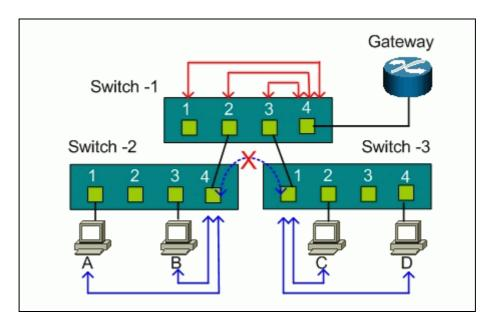
For Switch-1, port 1, port2, and port 3 are allowed to communicate back and forth with uplink port 4, but not with other ports.
