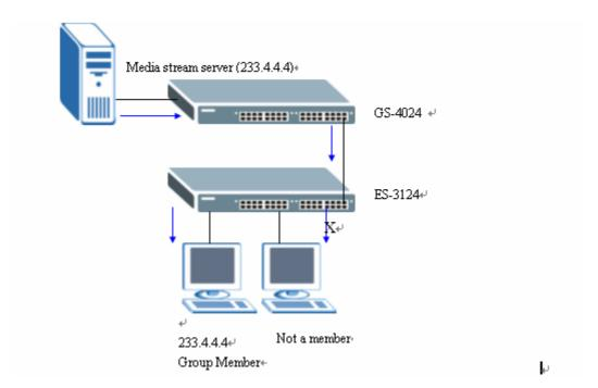
**Step one**: In the GS-4024, click the **IP Application**, select **IGMP** where, IGMP function can be enabled and we can select either IGMP-v1 or IGMP-v2.
