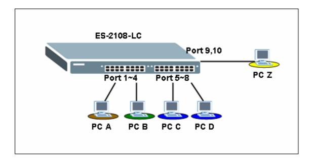
In this scenario, Port Based VLAN is used to separate one physical Switch into two smaller logical Switches. Port 1~4 and 9, 10 are in one group. And Port 5~10 are in another group. Port-based VLANs are specific only to the switch on which they were created.
