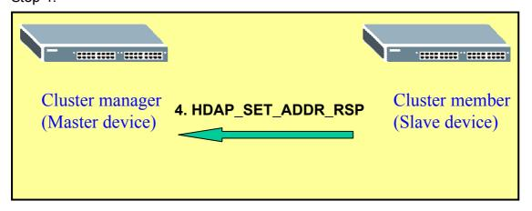
HDPA\_SET\_ADDR\_RSP (Slave device) packet response is for a clustering member to acknowledge a "Set Address" request. The hardware address uniquely identifies the sender of this response.
