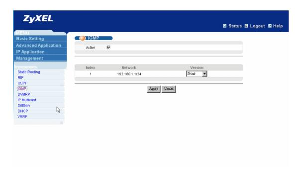
**Step two:** In the L2 Switch, click **Basic Setting** and then **Switch Setup** where we can enable IGMP snooping function with WEB-GUI.
