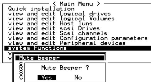
When the controller’s beeper has been activated, choose “Mute beeper,” then press **[ENTER]**. Choose “**Yes**” and press **[ENTER]** in the next dialog box to turn the beeper off temporarily for the current event. The beeper will still be activated on the next event.
