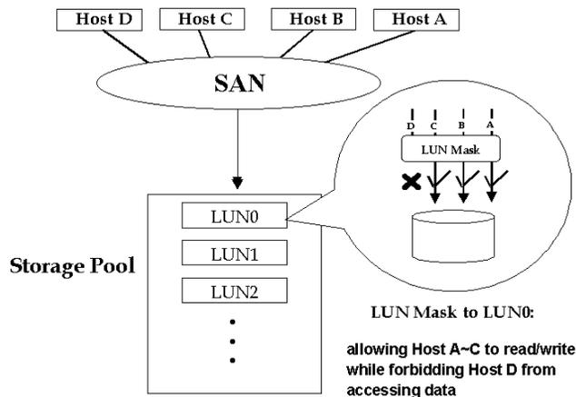
The access control can also be implemented by filter drivers. However, comparing to the control by software, access control based on controller LUN mapping can avoid overheads on server and the additional I/O latency. The LUN map combines **Host ID** (in the Fibre case, a 64-bit "port name;" in the SCSI case, the **initiator ID**) with the list of attributes of a LUN map that originally only consisted of the channel, target ID, and the LUN number.
