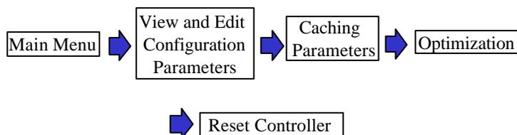
The controller optimization mode can only be changed when there is no existing logical configurations. Once the controller optimization mode is set, the same mode will be applied to all logical drives. Data stripe size is changed once the optimization method is changed. Therefore, you can not proceed with changing the optimization mode until data is backed-up, all logical drives deleted, and system restarted. Therefore, think twice before choosing an optimization mode for your controller.
