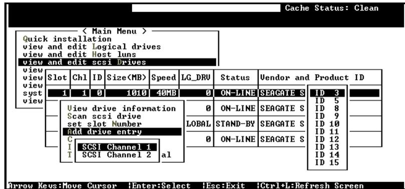
When there is an empty drive canister which currently does not contain any drive, the corresponding SCSI channel/ID will not appear in the drive information list. Assign a slot number to this empty canister and add a drive entry in order to use it later when a drive is installed.
