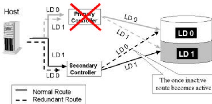
For every channel that is actively serving I/Os, there is another on the alternate controller that stays idle and will inherit the task should its counterpart fail.
