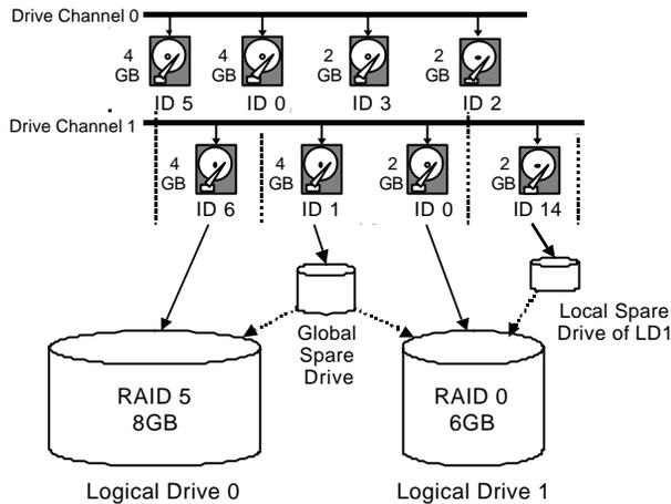
While grouping physical drives together, another drive can be assigned as the **Local Spare Drive** to one specified logical drive, or as the **Global Spare Drive**. A Local Spare is taken to rebuild one logical drive while a Global Spare participates in the rebuild of any logical drive in a RAID system.
