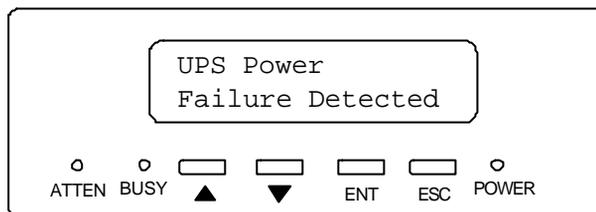
When the Fault-bus function is enabled and a failure signal is detected, an alert message will be shown on the LCD. The ATTEN LED will also light at the same time.
