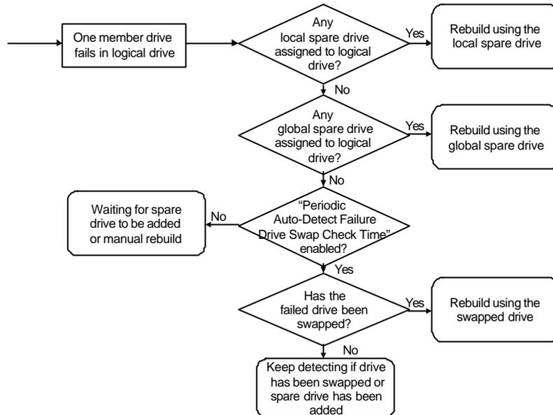
**Rebuild with Spare:** When a member drive in a logical drive fails, the controller will first examine whether there is a Local Spare Drive assigned to this logical drive. If yes, it will automatically start to rebuild.
