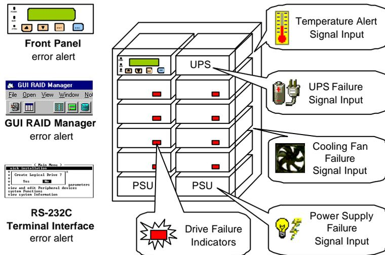
Fault-bus is actually a signal bus which contains a group of input and output signals. The Fault-bus design is fully open for easy integration. Simply install, configure and integrate the RAID controller with the enclosure, the RAID controller will be able to provide corresponding alert to the user for an immediate dispose to protect the data stored in the RAID system.
