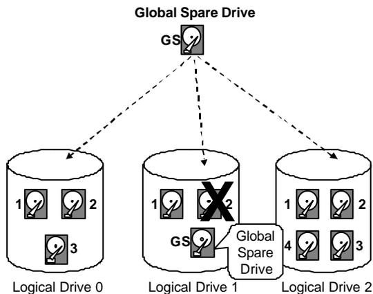
The external RAID controllers provide both Local Spare Drive and Global Spare Drive functions. On certain occasions, applying these two functions together will better fit various needs. Take note though that the **Local Spare Drive always has higher priority than the Global Spare Drive.**
