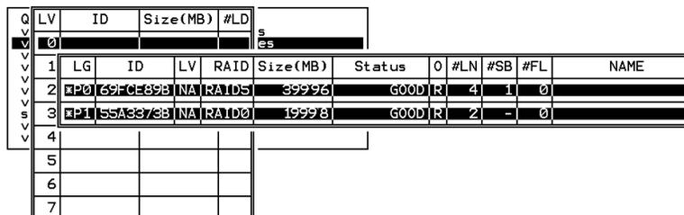
Select one or more logical drive(s) available on the list. The same as creating a logical drive, the logical drive(s) can be tagged for inclusion by positioning the cursor bar on the desired drive and then press **[ENTER]** to select. An asterisk (\*) will appear on the selected drive. Press **[ENTER]** again will deselect a logical drive.
