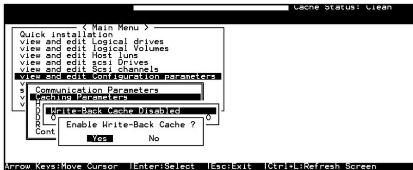
Choose “Caching Parameters”, then press **[ENTER]**. Select “Write-Back Cache,” then press **[ENTER]**. “Enabled” or “Disabled” will display the current setting with the Write-Back caching. Choose **Yes** in the dialog box that follows to confirm the setting.
