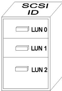
A SCSI channel (SCSI bus) can connect up to 15 devices (not including the SCSI controller itself) when the Wide function is enabled (16-bit SCSI). It can connect up to 7 devices (not including the controller itself) when the Wide function is disabled (8-bit SCSI). Each device has one unique SCSI ID. Two devices owning the same SCSI ID is not allowed.
