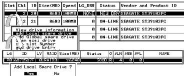
The screenshot shows a RAID controller interface with a menu and a table. The menu options are: View drive information, Add local spare drive, Add Global spare drive, Assign SCSI drive, Set slot Number, and Exit drive Entry. The table below shows logical drive information:
