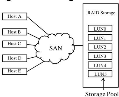
RAID-based mapping provides the centralized management for host-storage access. It is derived from the concept that storage can be divided into manageable pieces by mapping storage to different Logical Unit Numbers (LUNs). The storage can then be managed in the context of a LUN map. We then append filtering mask(s) to the LUNs making specific storage unit accessible or inaccessible to one or multiple host adapters.
