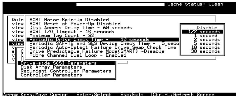
2. In \View and Edit Configuration Parameters\Drive-side SCSI Parameters\Drive Predictable Failure Mode <SMART>, choose one from "Detect Only," "Detect, Perpetual Clone" and "Detect, Clone+Replace."
