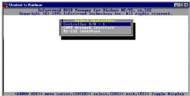
Execute the Text RAID manager program and select "Controller Maintenance." Press **[ENTER]** to proceed and then select "Upload NVRAM" as a file or "Download NVRAM" from a previously saved file.
