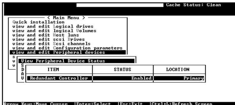
When the scanning has completed, the status will change to "Enabled."
