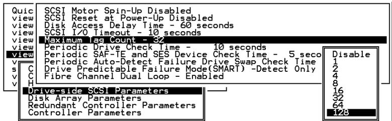
The controller supports tag command queuing with an adjustable maximum tag count from 1 to 128. The default setting is “Enabled” with a maximum tag count of 32. This setting can be changed or tag command queuing can be disabled. Choose “Maximum Tag Count”, then press **[ENTER]**. A list of available tag count numbers will appear. Move the cursor bar to a number, then press **[ENTER]**. Choose **Yes** in the dialog box that follows to confirm the setting.
