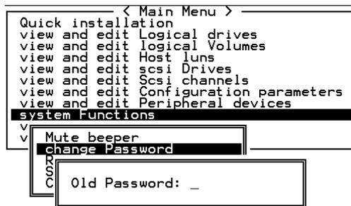
Use the controller's password to protect the array from unauthorized entry. Once the controller's password has been set, regardless of whether the front panel, the RS-232C terminal interface or RAIDWatch Manager is used, the user can only configure and monitor the RAID controller by providing the correct password.
