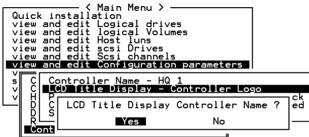
Choose "View and Edit Configuration Parameters," "Controller Parameters," then press [ENTER]. Choose to display the embedded controller logo or any given name on LCD. Giving a specific name to controller will help if you choose to configure a multiple number of RAID systems remotely through management software.
