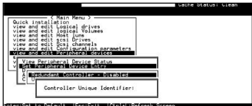
A Controller Unique Identifier is **required** for operation with the **Redundant controller configuration**. The controller will automatically notify users to enter a unique identifier when the first logical drive is created in a dual-controller system.
