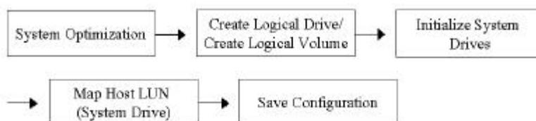
Drives must be configured and the controller properly initialized before host computer can access the storage capacity.
