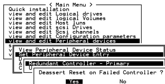
If the replacement has been initialized normally, you may proceed to examine the system status. From the main menu, select "View and Edit Peripheral Devices" and then "View Peripheral Device Status" to see that the new controller is being scanned.
