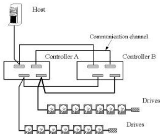
The physical connection between controllers should be similar to the one shown above. All channels should be connected to both controllers. The path default for controller communications (SCSI) is channel 0. Channel 0 is also the default for host interface; therefore, avail other channel for host connection by changing its channel mode.
