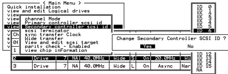
Choose a Drive channel, then press **[ENTER]**. Choose “Secondary Controller SCSI ID.” A list of SCSI IDs will be displayed on the screen. Assign a SCSI ID to the drive channel of the secondary controller. Choose a SCSI ID. The dialog box “Change Secondary Controller SCSI ID?” will appear. Select **Yes**, then press **[ENTER]**.
