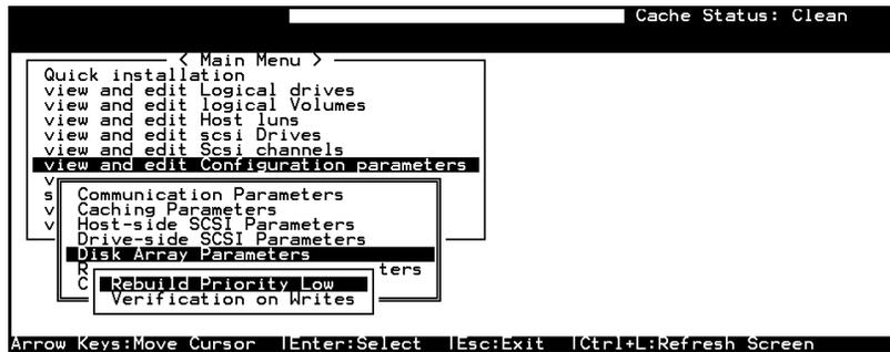
Select “View and edit Configuration parameters” on the main menu and press **[ENTER]**. Choose “Disk Array Parameters,” then press **[ENTER]** again. The Disk Array Parameters menu will appear.
