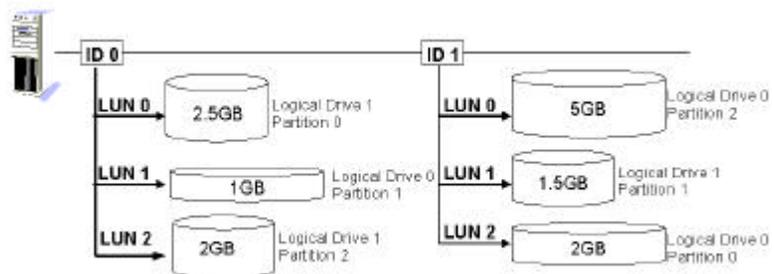
Map each partition to LUNs under host SCSI IDs or IDs on host channels. Each SCSI ID/LUN will act as one individual hard drive to the host computer virtually. In this way, estimated workload can also be distributed over different data paths for performance optimization.
