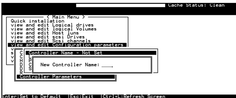
Choose "View and Edit Configuration Parameters," "Controller Parameters," then press [ENTER]. The current controller name will be displayed. Press [ENTER]. Enter the new controller name in the dialog box that follows, then press [ENTER].
