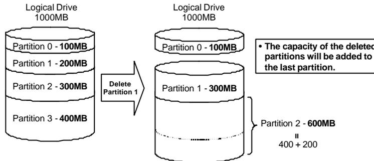
As illustrated above, the capacity of the deleted partition will be added into the last partition.
