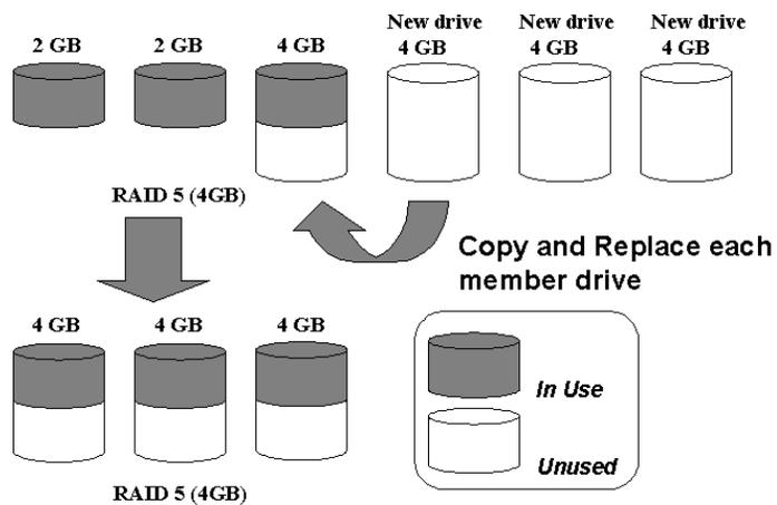
*After all the member drives have been replaced, execute the “Expand logical drives” to make use of the unused capacity.*
