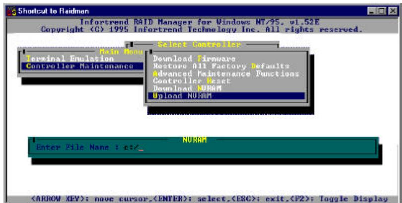
Provide location and file name, then press **[ENTER]** to proceed. The uploading or downloading process will be completed almost instantly.
