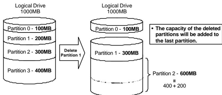
The capacity of the deleted partition will be added to the last partition.
