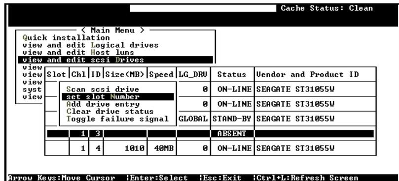
Move the cursor bar on the empty drive entry and press **[ENTER]**. Choose “Set Slot Number” in the menu, then press **[ENTER]**. Enter the slot number of this empty canister so as to use it later when a drive is installed.
