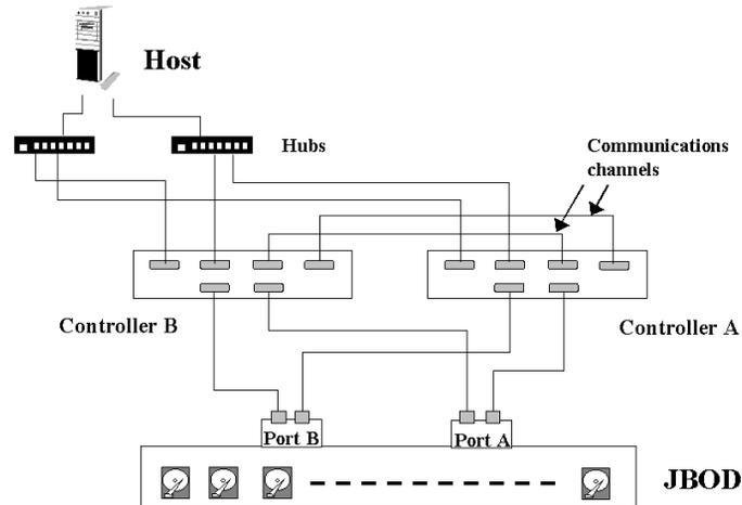
With Fibre-to-Fibre controllers, there are basically three choices with inter-communications:
