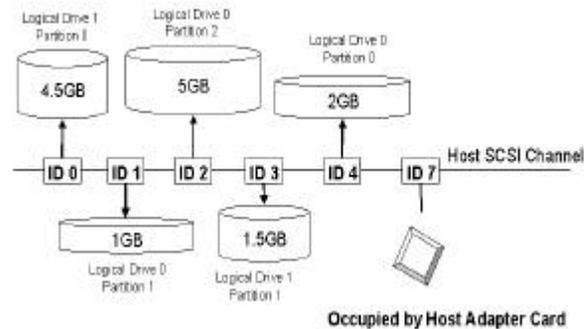
Some operating systems do not read multiple LUNs under single SCSI ID. As diagrammed above, you may create multiple IDs on the host channel and map logical configurations to these IDs. Each of these IDs can be designated as Primary or Secondary. Units mapped to Primary IDs will be managed by the Primary controller, and those mapped to Secondary IDs Secondary controller. As a rule, each unit will be mapped to LUN0 under each SCSI ID.
