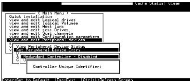
Controller Unique Identifier is **required** for operation with the **Redundant controller configuration**. The controller will automatically notify users to enter a unique identifier when the first logical drive is created in a dual-controller system.
