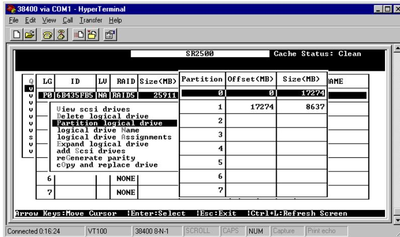
Follow the directions in chapter 6 and chapter 8 to map the new partition to a Host LUN. The new partition must be **"mapped"** to a host LUN in order for the HBA (host-bus adapter) to see it. Once you have mapped the partition, reboot Windows NT. The HBA should be able to detect an additional "disk" during the initialization process.
