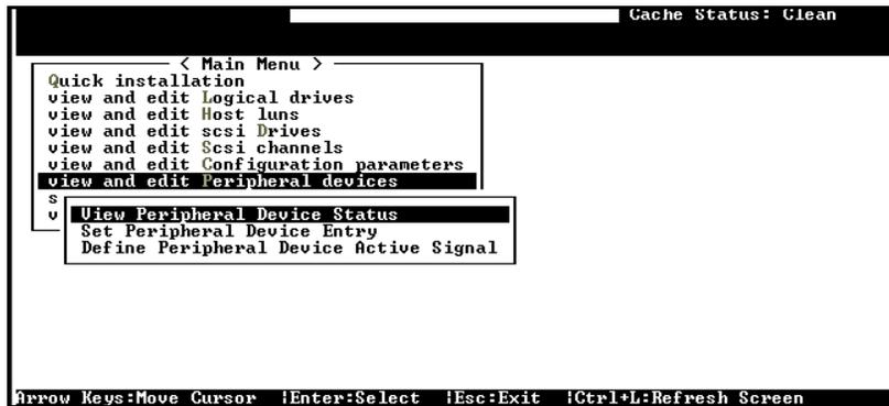
Choose “View and Edit Peripheral Devices” in the Main Menu and press **[ENTER]**. Select “View Peripheral Device Status” in the menu and press **[ENTER]**.
