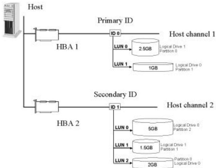
configuration of drives to LUNs under either ID and thus divide or distribute the workload specifically to different controllers.
