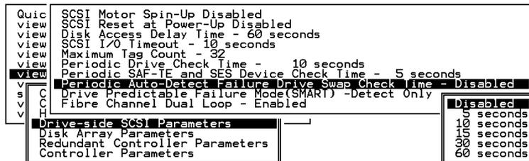
Choose “Periodic Drive Check Time;” then press [ENTER]. Move the cursor to the desired interval; then press [ENTER]. Choose **Yes** in the dialog box that follows to confirm the setting.
