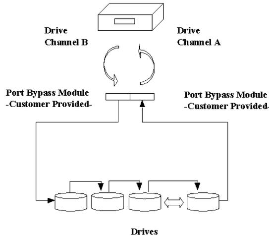
Controller firmware will automatically examine the node names and port names of all the connected drives once initiated. If devices on two different drive channels appear with the same loop ID and port name, controller will consider these two drive channels as a "dual loop."
