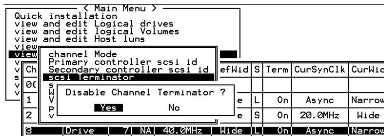
Choose the channel you wish the terminator enabled or disabled, then press **[ENTER]**. Choose “SCSI Terminator”, then press **[ENTER]**. A dialog box will appear. Choose **Yes**, then press **[ENTER]**. Terminator can also be enabled by switch jumpers, please refer to the controller hardware manual for more details.
