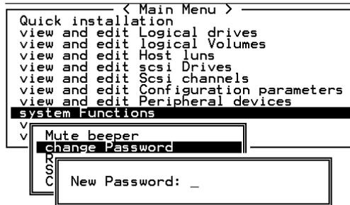
Enter the desired password in the column, then press **[ENTER]**. The next dialog box will display “Re-Enter Password”. Enter the password again to confirm and press **[ENTER]**.
