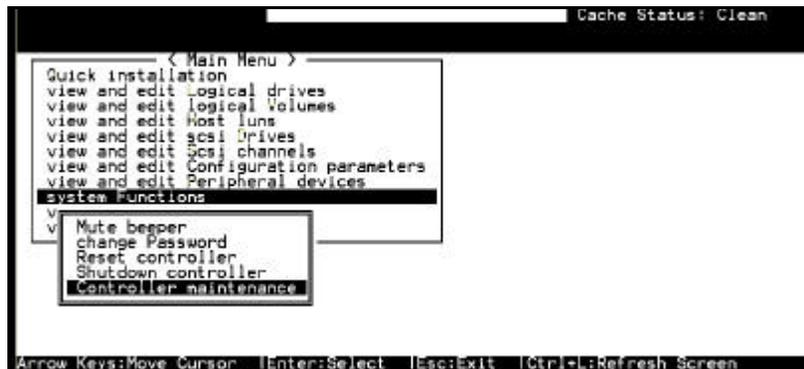
Choose “System Functions” in the main menu, then press **[ENTER]**. The System Functions menu will appear. Move the cursor bar to an item, then press **[ENTER]**.
