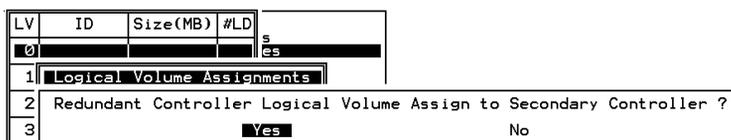
Logical volumes can also be assigned to different controllers (primary or secondary). Default is primary. Press **[ESC]** if change is not preferred.
