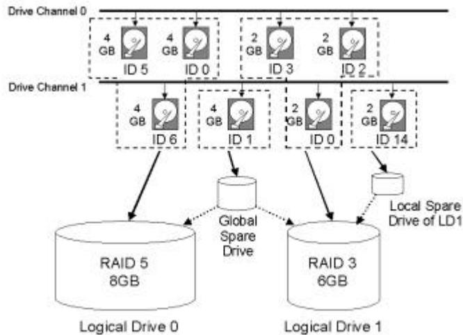
A drive can be assigned as the Local Spare Drive to one specified logical drive, or as a Global Spare Drive. Spares can be conducted to automatic system rebuild. Spare is not available for logical drives that has no data redundancy (NRAID and RAID 0).
