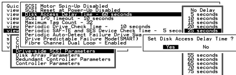
Choose “Disk Access Delay Time,” then press **[ENTER]**. A list of selections will appear. Move the cursor bar on a selection, then press **[ENTER]**. Choose **Yes** in the dialog box that follows to confirm the setting.
