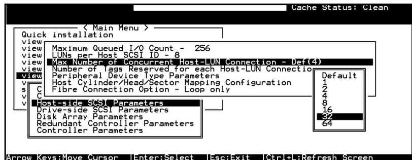
From the main menu, select “View and Edit Configuration Parameters,” “Host-side SCSI Parameters,” then press [ENTER]. Choose “Max Number of Concurrent Host-LUN Connection,” then press [ENTER]. A list of available selections will appear. Move the
