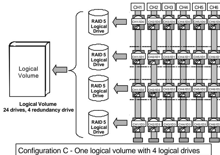
As illustrated above, should one of the drive channels fail, each logical drive loses one of its members. Logical drives will still be capable of normal operation. Data remains intact and the rebuild can be performed after the failed channel is recovered. No access interruptions to the logical volume will be experienced on the host side.
