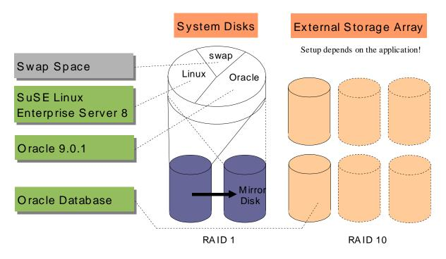
The hardware consists of two main systems: A computer system (the server) with one or better two internal disks and a hardware RAID controller, and an external storage unit with lots of space, typically connected via an external SCSI cable or a fiber channel cable (more robust).
