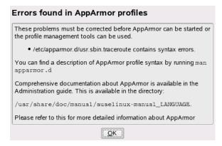
To fix a syntax error, log in to a terminal window as root, open the profile, and correct the syntax. Reload the profile set with rcapparmor reload.
