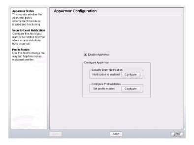
From the *AppArmor Configuration* screen, determine whether Novell AppArmor and security event notification are running by looking for a status message that reads *enabled* or configure the mode of individual profiles.
