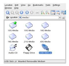
You can also name removable devices, such as USB sticks, with Konqueror. Right-click the USB stick in Konqueror and select *Properties*. On the *General* tab, enter a name in the input field and click *OK*. When inserting the stick the next time, Konqueror displays the name of the stick.
