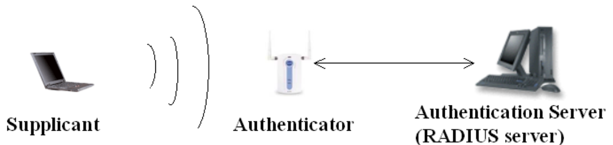
Fig. IEEE 802.1X w/ Standalone RADIUS server
