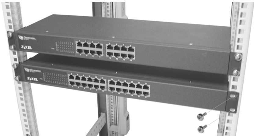
Figure 2-3 Mounting the ES to an EIA standard 19-inch rack
