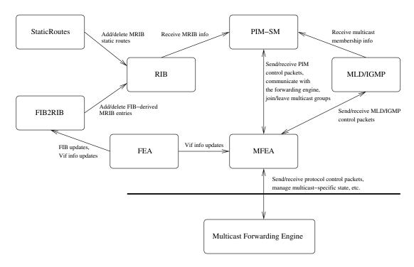
Figure 2: Multicast Modules Interaction
