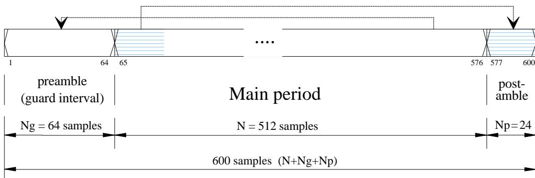
Figure 4: OFDM symbol structure. Samples of the main period are repeated for pre- and postamble.
