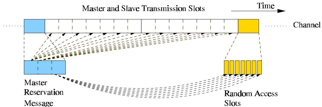
Figure 2: Structure of a master-slave type access protocol
