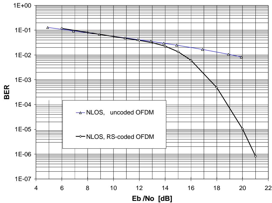
*Figure 11: Uncoded and coded bit error rates of the overall MEDIAN physical layer for a Non Line of Sight (NLOS) multipath channel (target environment for future system). HPA nonlinearities, LO phase noise, synchronisation are included.*
