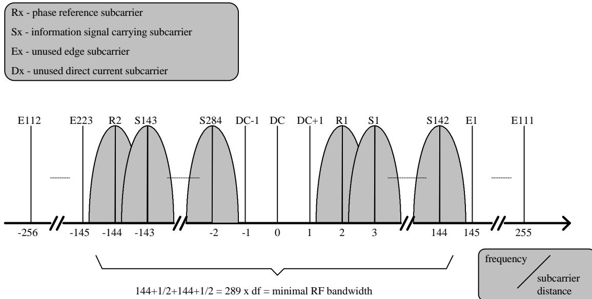
Figure 3: OFDM subcarrier allocation (frequency spectrum) in the equivalent lowpass domain.
