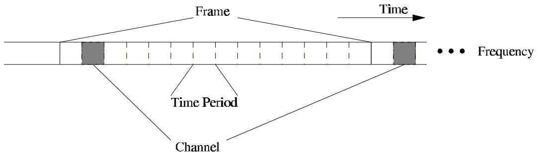
Figure 1: Definition of a channel
