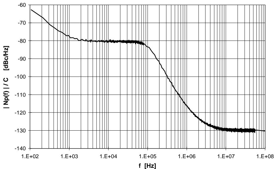
*Figure 7: Phase noise mask of 56GHz local oscillator to be used in the MEDIAN demonstrator (approximated PSD curve based on measurements by Dassault Electronique)*
