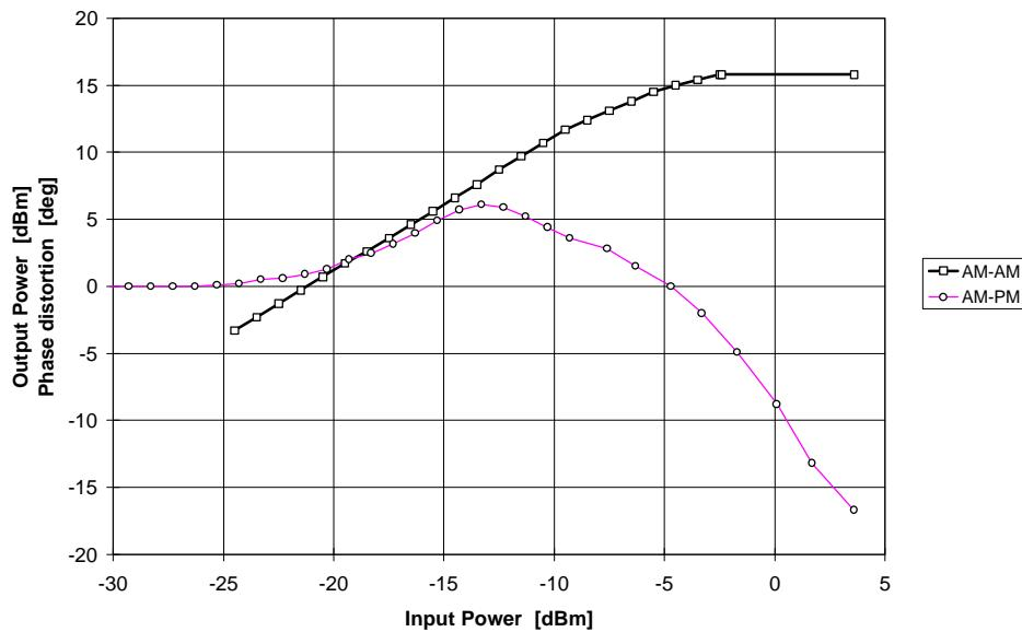
Figure 6: AM-AM and AM-PM conversion of 60GHz high power amplifier (HPA) to be used in the MEDIAN demonstrator (model based on measurements by Dassault Electronique)
