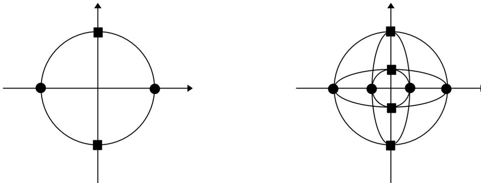
Fig. 1: Trajectories of MSK/OQPSK and OQAM
