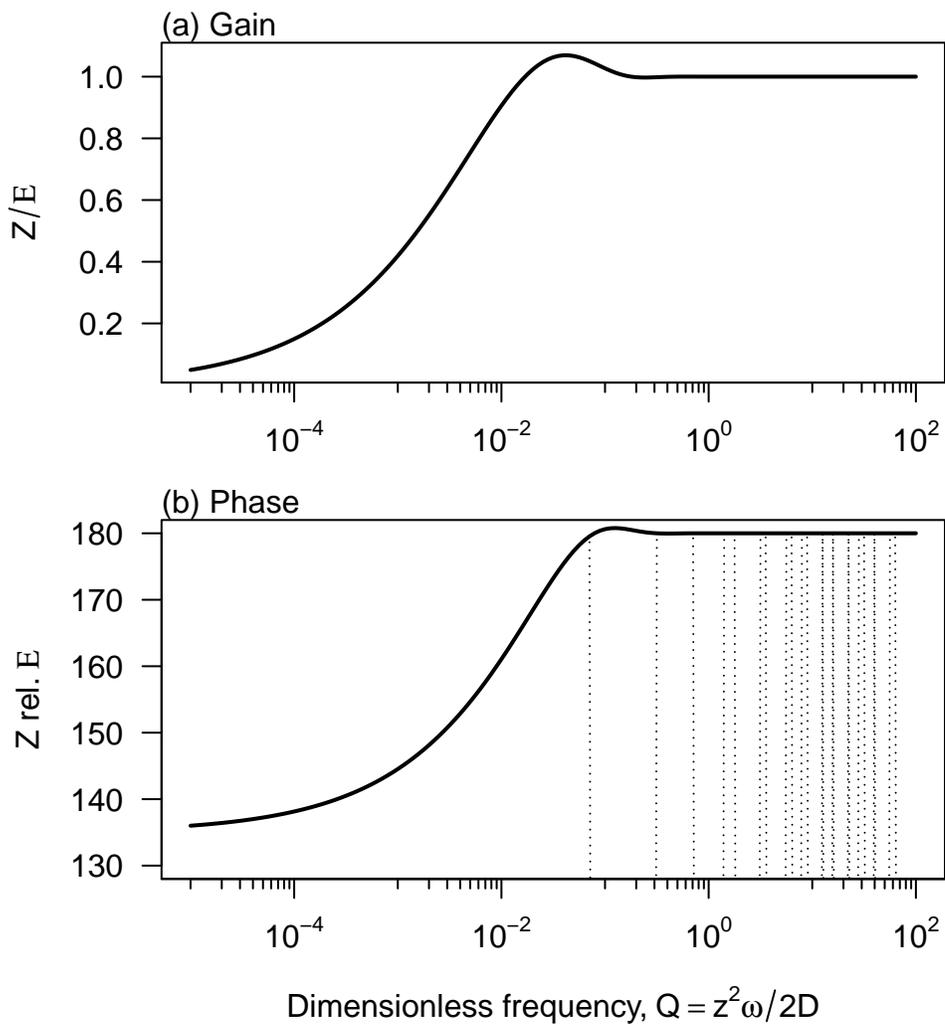
**Figure 5:** The response of an open well to harmonic areal strain using the Rojstaczer model. Modified from Rojstaczer (1988, Fig. 3). Frequency is dimensionless, based on the well-depth  $z$  and the diffusivity  $D$ .
