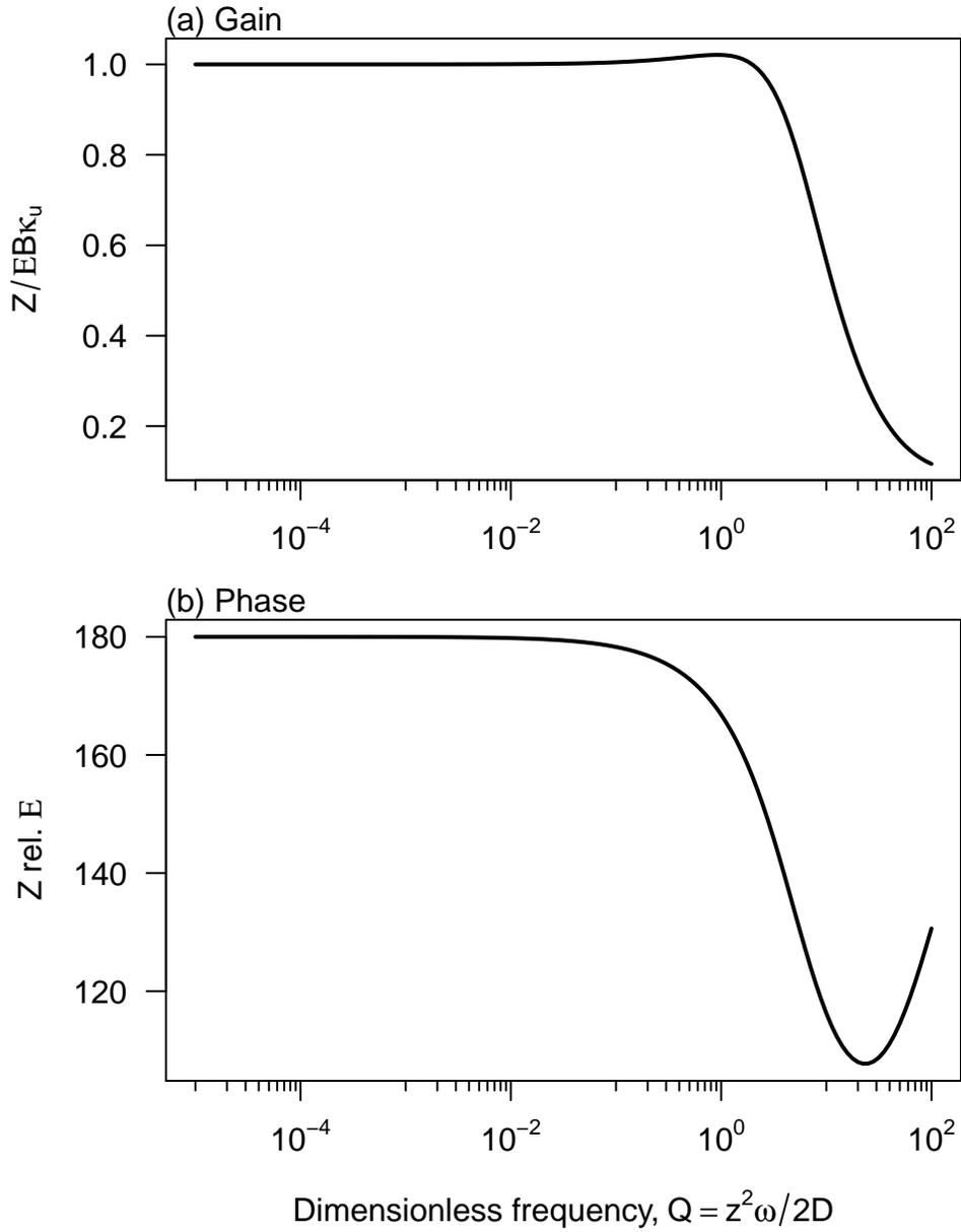
**Figure 1:** The response of a sealed well to harmonic areal strain using the Kitagawa model. The amplitude is normalized by Skempton's coefficient  $B$  and the undrained bulk modulus  $\kappa_u$ . Frequency is dimensionless, based on the well-depth  $z$  and the diffusivity  $D$ .
