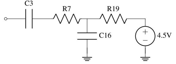
Figure 3: Klon Centaur Feed-Forward Network 1 Circuit
